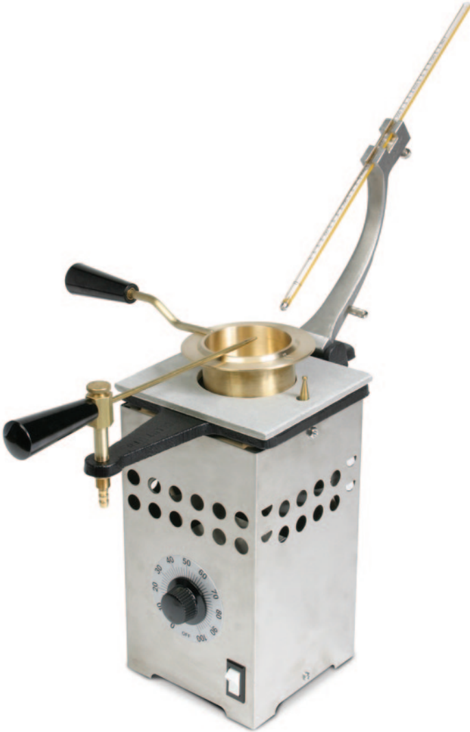
Cleveland Flash & Fire Point Tester
