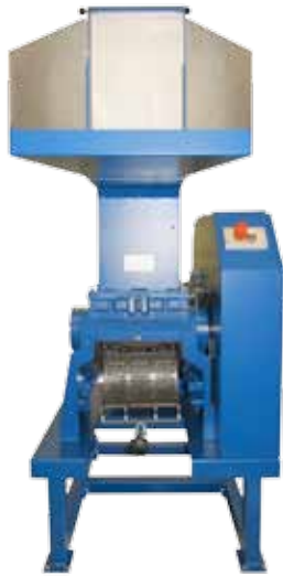
Cutting Mill with closed „EASY LOCK COVER“
