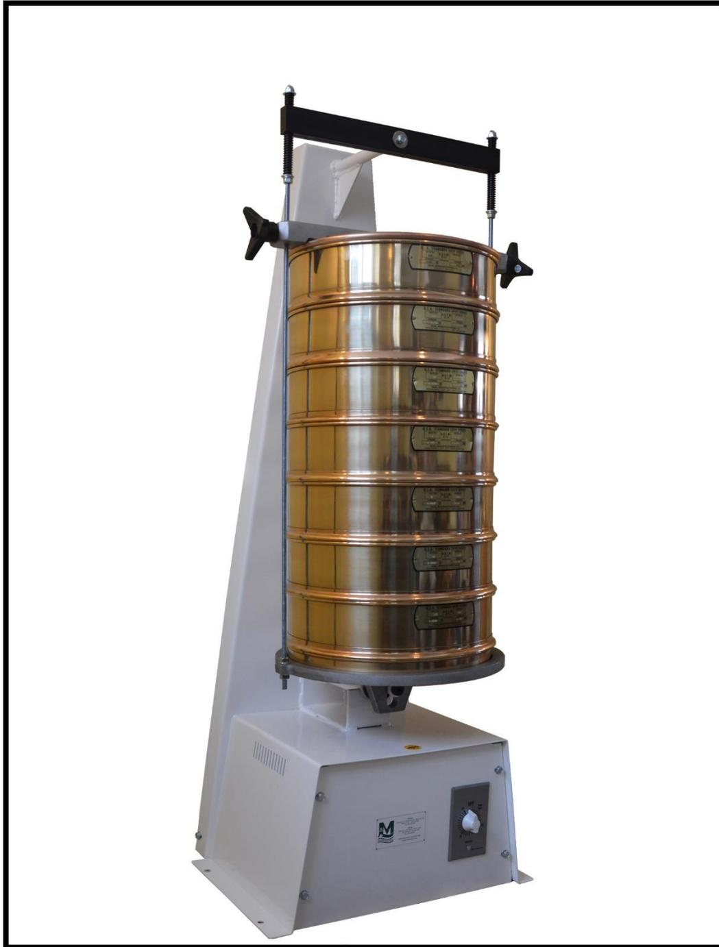
Thank you for purchasing the ML4330 sieve shaker. You and your company will have many years of use from this quality testing system. This sieve shaker has the ability to accommodate a variety of sieves from 8 inch up to 12 inch diameter or metric equivalent.
